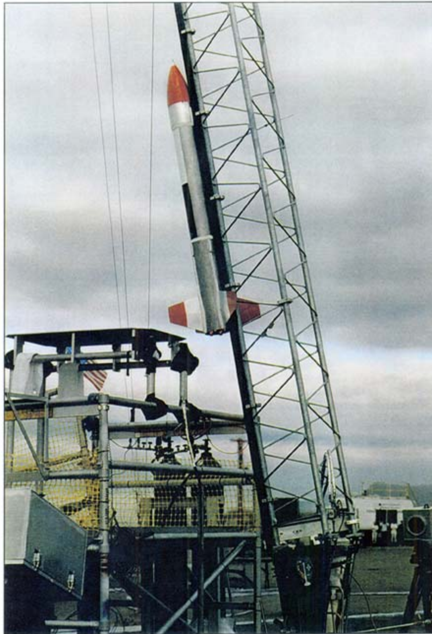
LLNL's pump-fed hydrazine rocket, ASTRID, ascends the launch rail on February 4, 1994 at Vandenberg. The 4 thrust chambers are glowing but the plume is invisible.
